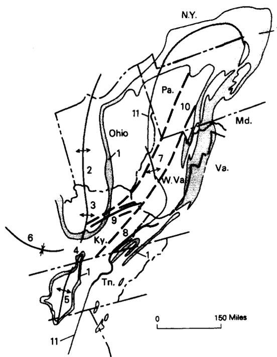
Fig. 12. Map showing structural elements and Devonian outcrop belt in the Appalachian Basin. (1) Devonian outcrop belt, (2) Cincinnati arch, (3) Jessamine dome, (4) Cumberland saddle, (5) Nashville dome, (6) Illinois Basin, (7) Burning Springs anticline, (8) Pine Mountain fault, (9) Kentucky River, Irvine–Paint Creek fault zone, (10) Rome trough, heavy dashed lines represent faults bounding the graben, (11) western limit of thrusting.
