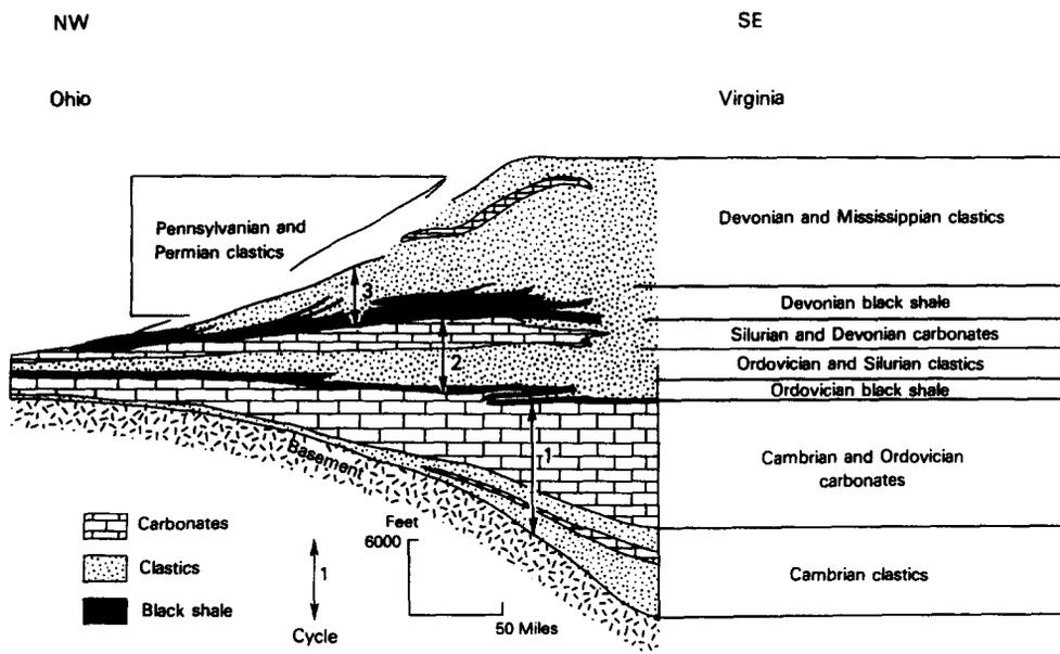
Fig. 2. Stratigraphic cross-section of the Appalachian Basin showing the cyclic relationship of the basin fill. The Devonian black shale is the basal sequence of cycle 3. Modified from Colton (1970).
