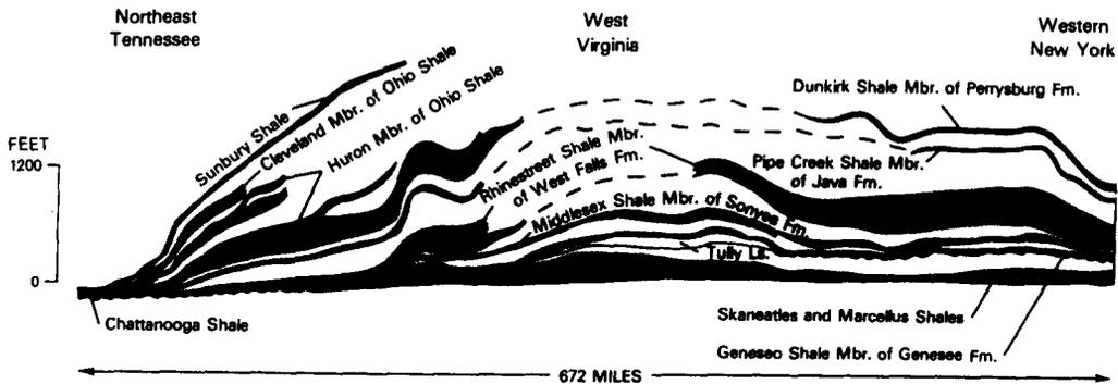
Fig. 5. Longitudinal cross-section through the central part of the Appalachian Basin showing the regional stratigraphic relationship of the Middle and Upper Devonian black shale units. In part diagrammatic. Modified from the center longitudinal cross-section shown in Fig. 1.
