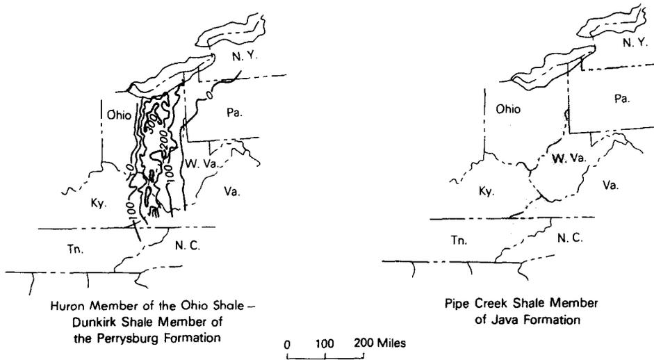
Fig. 8. Isopach map of the Huron Member of the Ohio Shale and its equivalent, the Dunkirk Shale member of the Perrysburg Formation; contour interval as shown, thickness in feet. Distribution of the Pipe Creek Shale Member of the Java Formation shown by shading.
