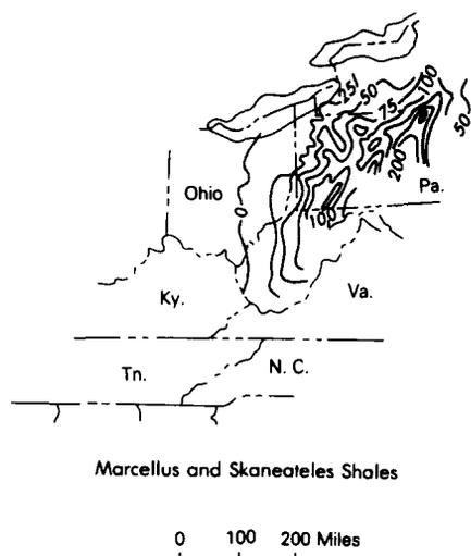
Fig. 11. Isopach map of the Marcellus and Skaneateles Shales, undivided; contour interval as shown, thickness in feet.
