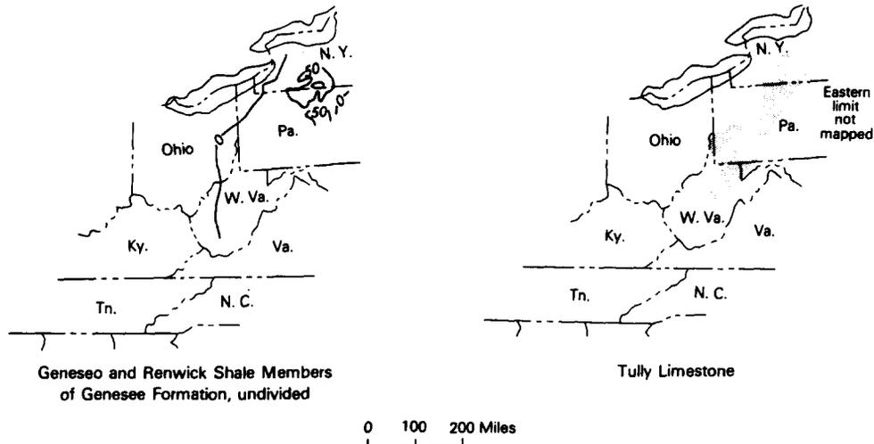
Fig. 10. Isopach map of the Genesee and Renwick Shale member of the Genesee Formation, undivided; contour interval as shown, thickness in feet. Distribution of the Tully Limestone shown by shading.
