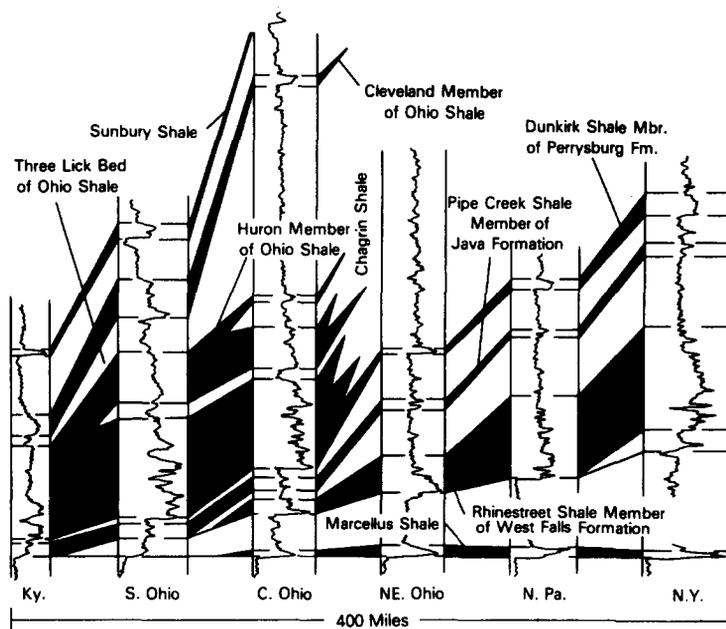
Fig. 6. Selected gamma-ray logs from the westernmost longitudinal cross-section (Fig. 1) illustrating long-distance regional correlations and characteristic log signature for black shale units.
