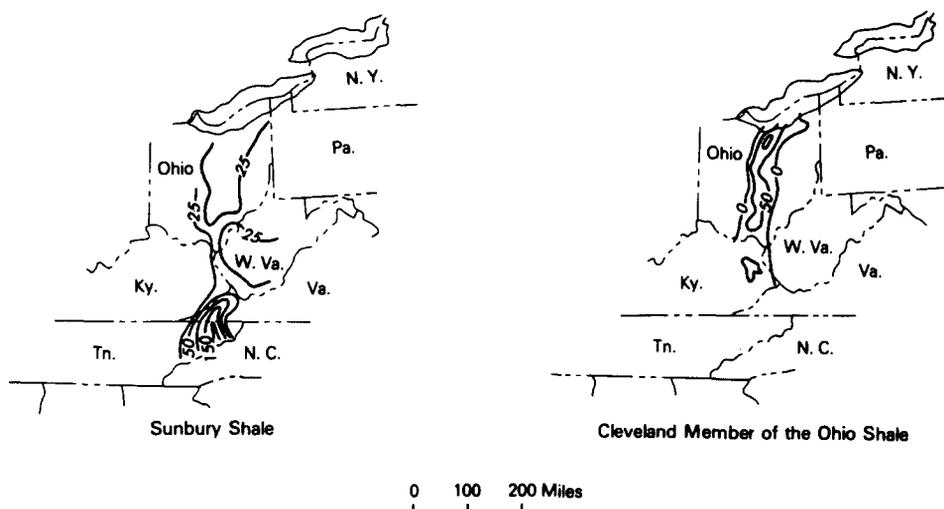
Fig. 7. Isopach map of the Sunbury Shale and the Cleveland Member of the Ohio Shale; contour interval as shown, thickness in feet.
