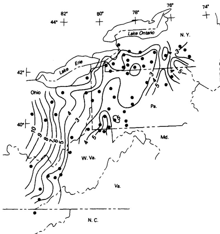
Fig. 3. Average organic carbon of the black shales of Middle and Late Devonian age (numbers and contours indicate %). Analyses from Claypool and Stone (1979), Claypool *et al.* (1980), Claypool (written communication, 1981) and Maynard (1981). Sample locations shown by black dots.
