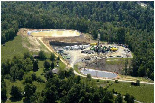
Water storage at a typical gas well
