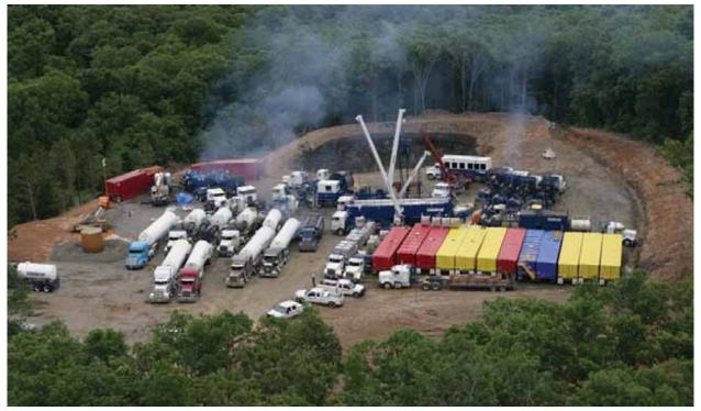
The numerous truck-mounted pumps and temporary storage tanks needed to fracture-treat the Marcellus Shale will require larger well locations. The fracturing equipment and materials on location in this photograph represent over 100 round trips to location by large tractor trailer trucks.
