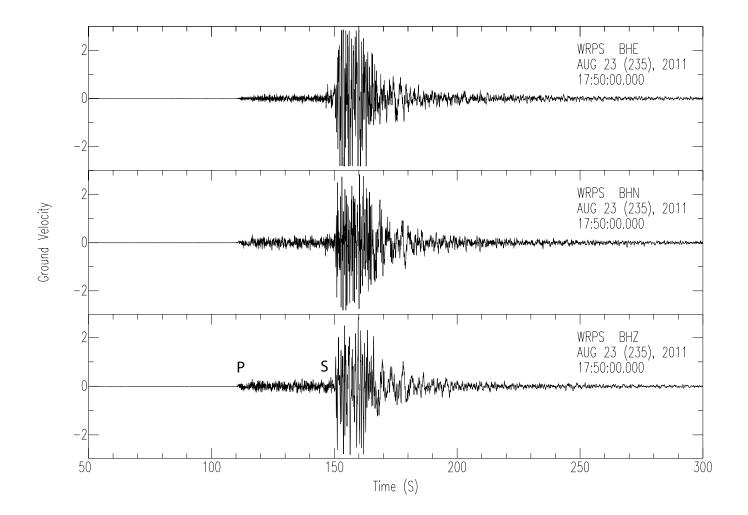
P and S waves are labeled. The largest amplitude S waves lasted for about 15 seconds .
